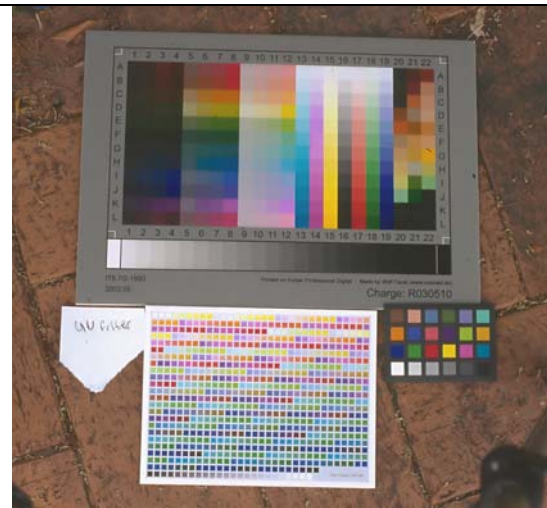
Figure 2: This picture demonstrates the change after hue and saturation colour corrections have been applied. The colour panels on the Colour checker are now accurately represented. The colour panels on the IT8 target have been validated as being close to the true colour.
