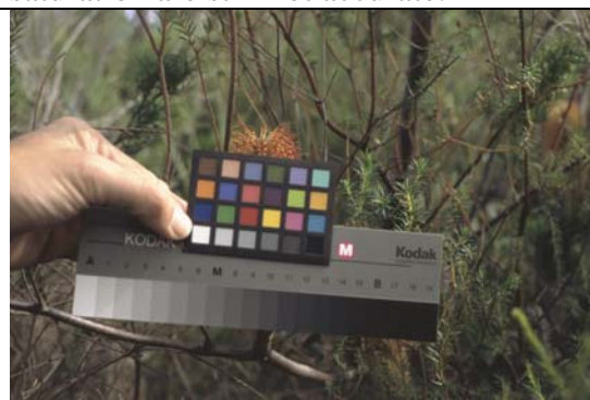
Figure 3: The technique applied to a photograph of Banksia ericifolia . The picture contains a Macbeth colour checker target. This picture has been rendered colour neutral, but without compensation for hue and saturation.
