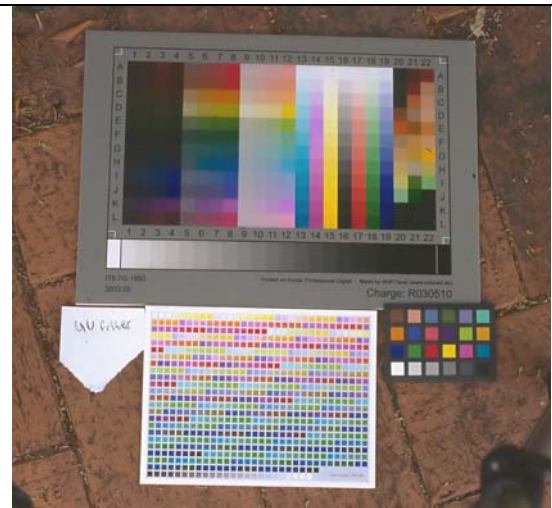
Figure 2: This picture demonstrates the change after hue and saturation colour corrections have been applied. The colour panels on the Colour checker are now accurately represented. The colour panels on the IT8 target have been validated as being close to the true colour.
