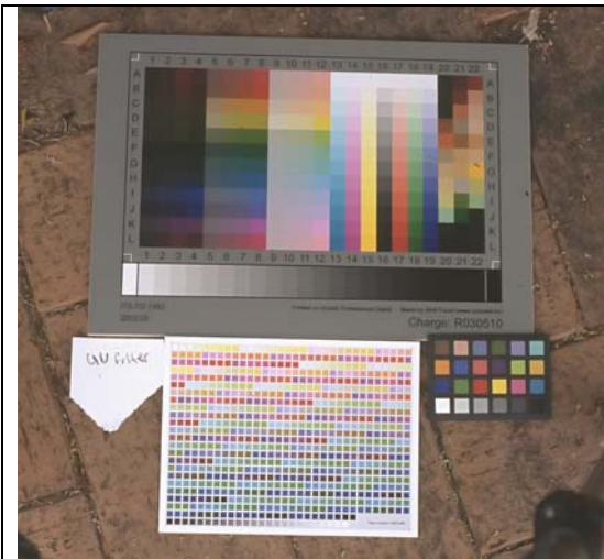
Figure 1: IT8 and Macbeth Colour checker targets. Pictures containing multiple targets were used to validate the technique. This particular slide demonstrates a picture that has been rendered colour neutral (eg, all of the grey patches are grey), but the hue and saturation are still not accurate.
