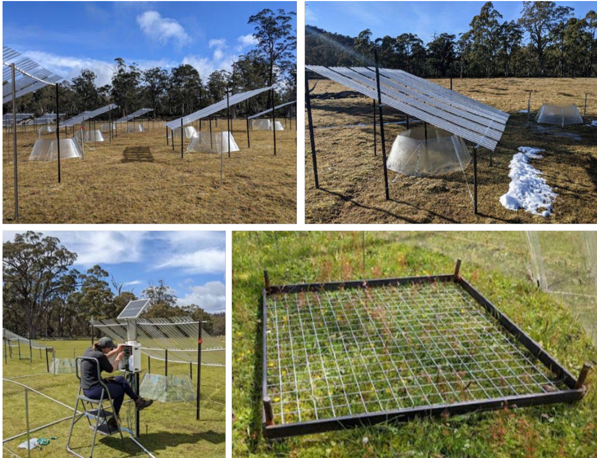
Top left and right: Drought shelters and warming chambers within the experiment. Bottom left: Wiring thermocouples and soil moisture sensors to datalogger, bottom right: Grid-frame secured into footings ready for compositional survey in a drought x warming plot. Images courtesy of Melissa Gerwin.
