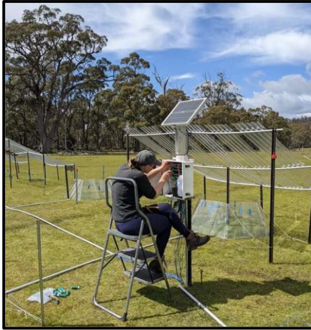
Figure 2 (left). Wiring thermocouples and soil moisture sensors to datalogger.
