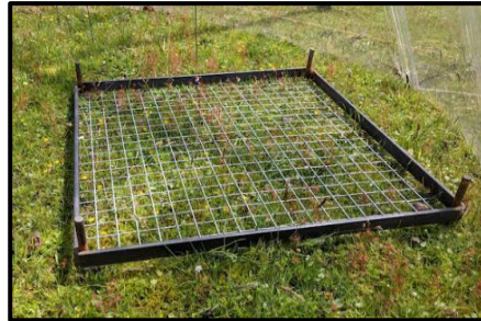
Figure 3 (below). Grid-frame secured into footings ready for compositional survey in a drought x warming plot.
