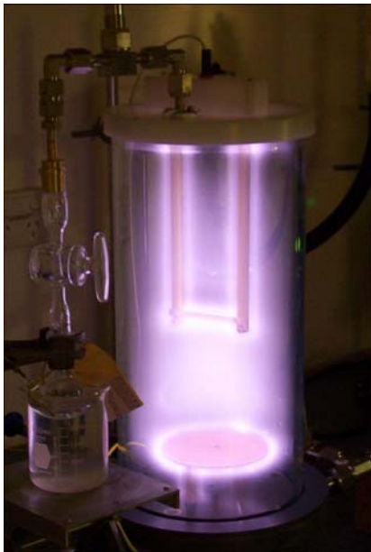
A gas plasma inside a glass chamber. The seeds are placed on the round table (diameter 90 mm).
